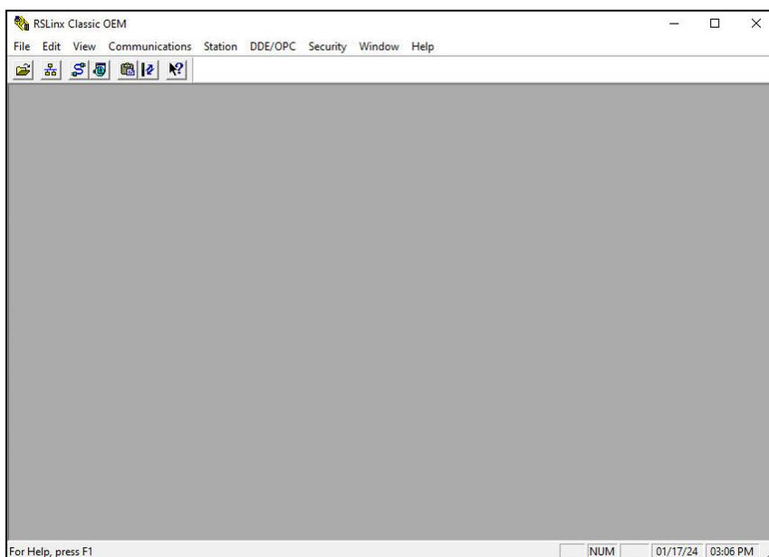
*Event Logger* assumes that the PLCs to be monitored are all on the same Ethernet network. Thus, RS Linx must first be configured to communicate with that network. This is accomplished by installing an Ethernet driver.
