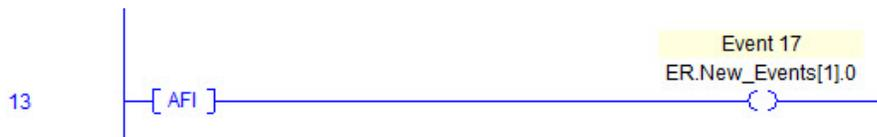
Replacing the AFI with a digital address or a digital condition will assign that address or condition associated Event address. Rungs must be added for more events to be monitored. Note that “ER.New\_Events” is a 16 bit integer array so that after bit 15 a new word with bit 0 is used.
